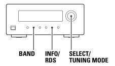
RDS is a broadcasting service which allows stations to send additional information along with the regular radio programme signal.
